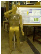
Hollow physical phantom in the Antenna Measurement Laboratory, Queen Mary, University of London, used for measurement protocol settings
