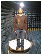
Microstrip patch antennas placed on the left waist (Tx) and right side of the chest (Rx) for 2.4 GHz on-body propagation measurement in the chamber
